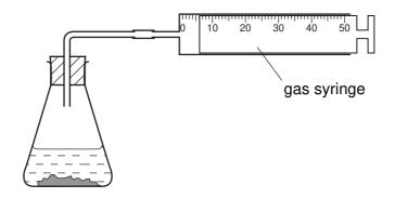
Solids **W** and **X** both catalyse the breakdown of hydrogen peroxide. The syringe diagrams show the volume of oxygen formed every 20 seconds using these catalysts at 25 °C.
